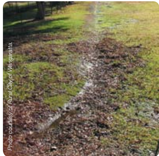
Boggy soil indicating a failing wastewater system.
